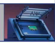
The hold-down system allows manual adjustment of the retaining (hold-down) positions in an x / y direction, thus ensuring individual alignments for each test specimen.
